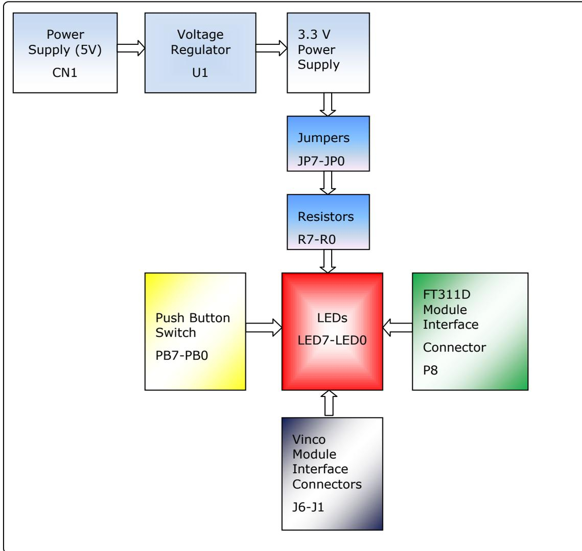
**Figure 2.1 : FT311 GPIO Board Block Diagram**
