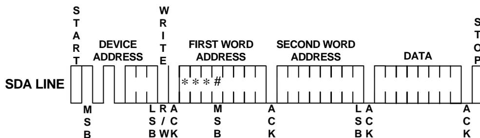
Figure 3: Byte Write
