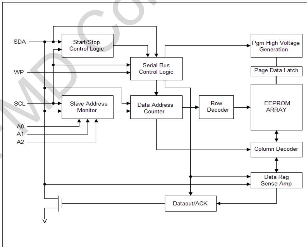
Figure 2: Block Diagram
