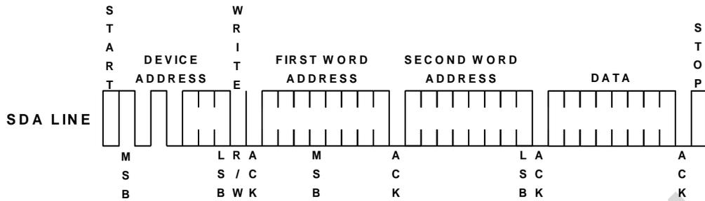
Figure 5: Byte Write
