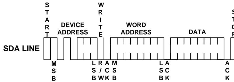
Figure 5: Byte Write
