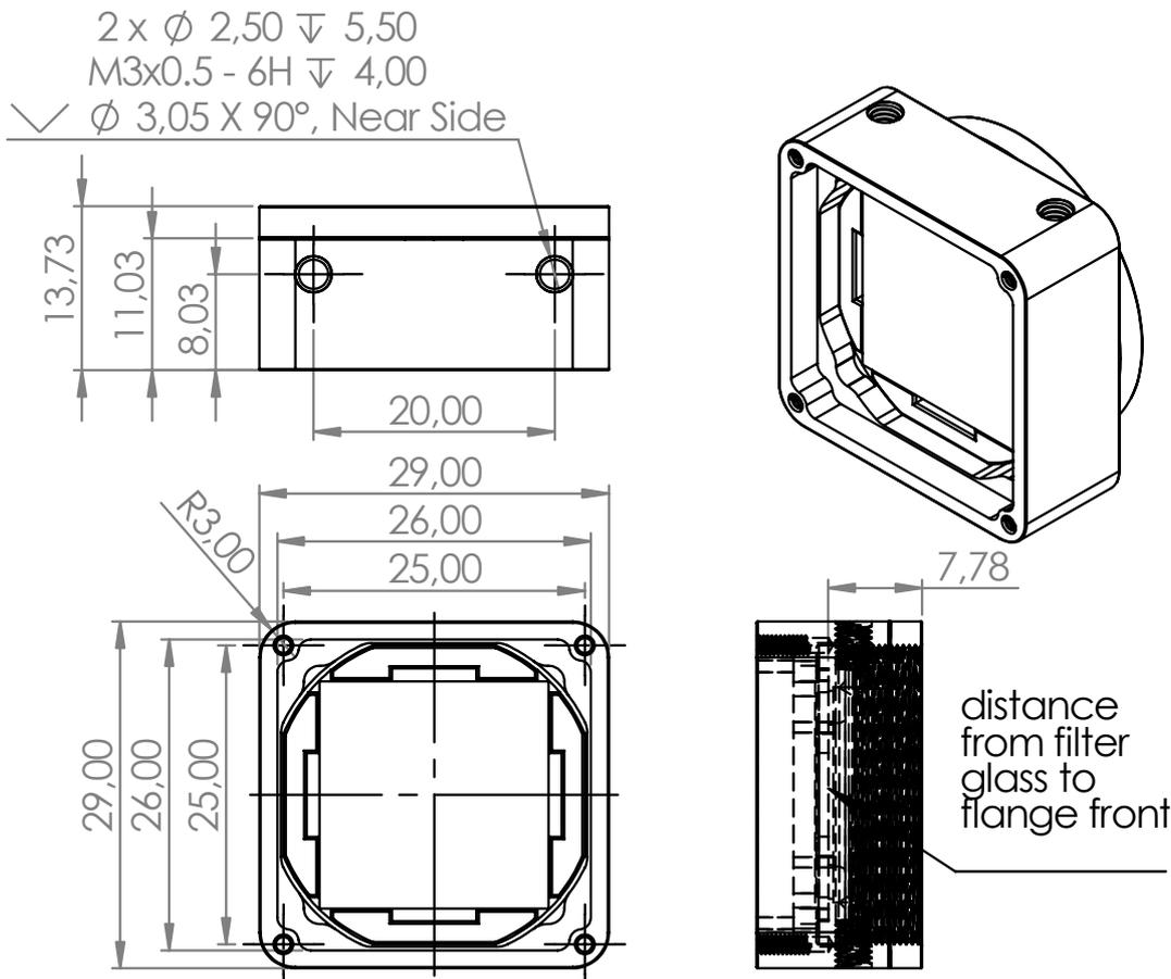
Figure 4: CS-Mount Body for 28 mm FSM
