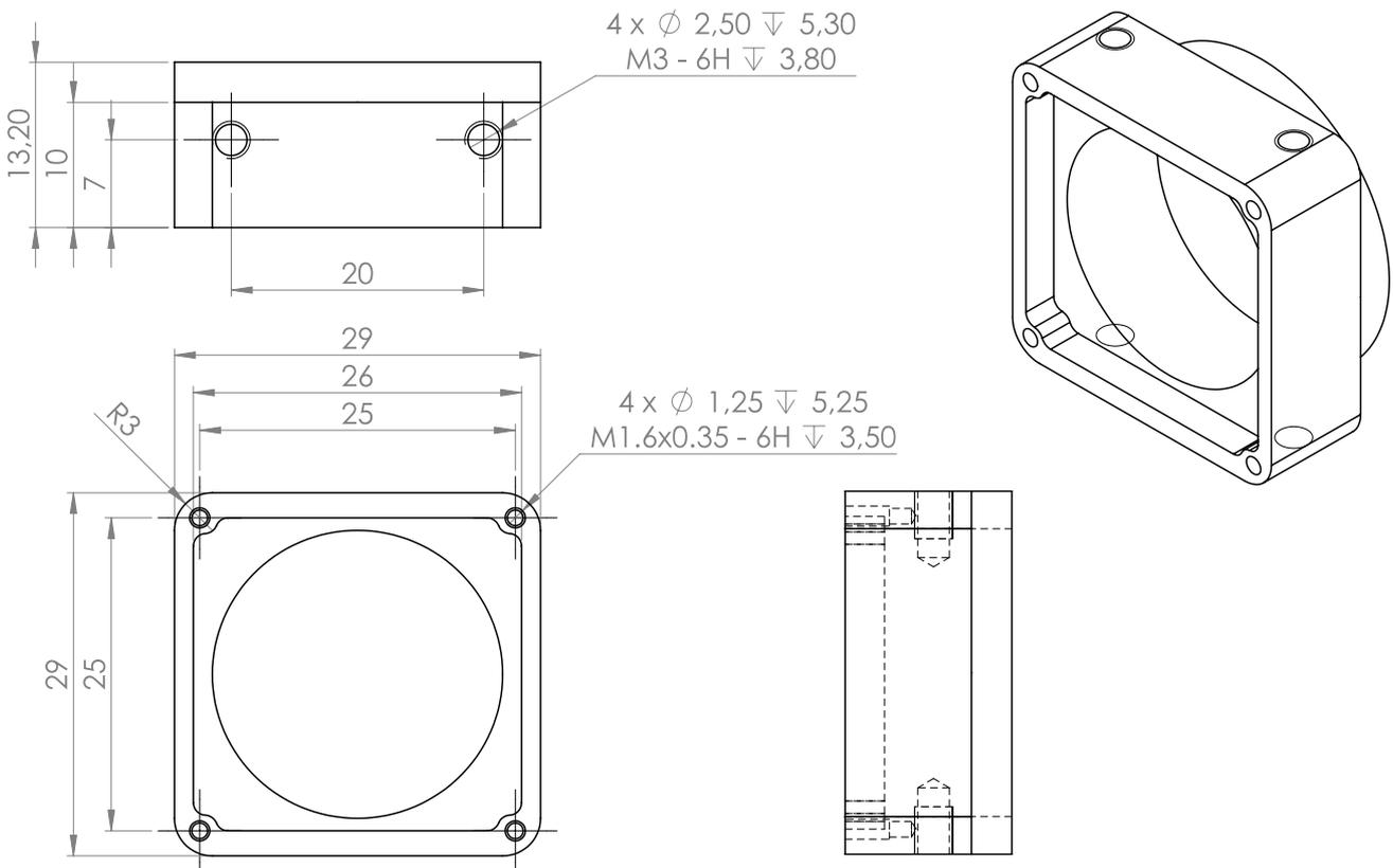
Figure 3: CS-Mount Body for 28 mm FSM
