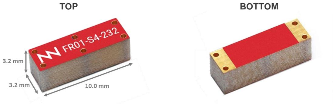
**Material:** The BAR mXTEND™ Antenna Booster is built on glass epoxy substrate.
