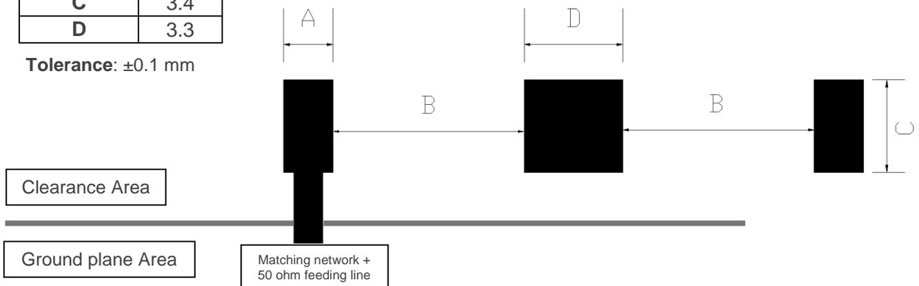
**Figure 10 – Footprint dimensions for the double booster.**
