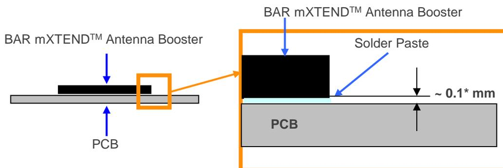
Figure 12 – Soldering Details.
