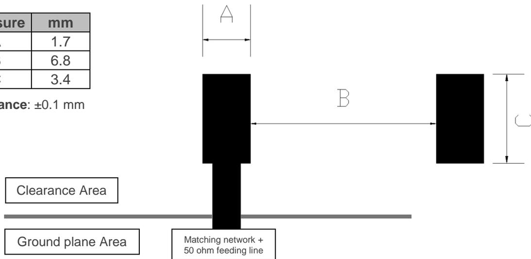
**Figure 9 – Footprint dimensions for the single booster.**
