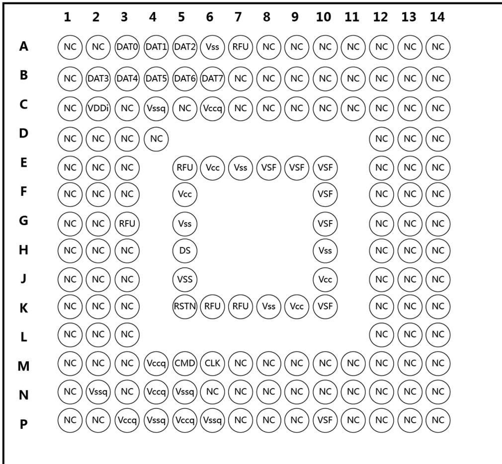
**FBGA153 - Ball Array (Top View through package)**
