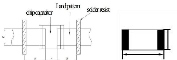
Recommended land dimensions for reflow-soldering (unit: mm)
