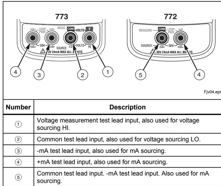
Figure 4. Input/Output Jacks
