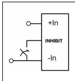
The products are fitted with a remote control function referenced to the primary negative input connection (- In), positive logic. The INHIBIT function allows the regulator to be turned on/off by an external device like a semiconductor or mechanical switch. The INHIBIT pin has an internal pull up resistor to + In.
