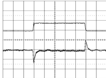
Output voltage response to load current step-
