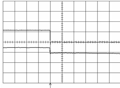
Shut-down enabled by disconnecting  $V_I$  at:
