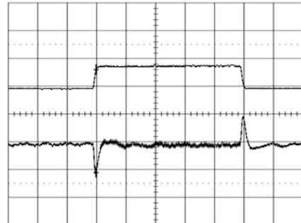
Output voltage response to load current step-
