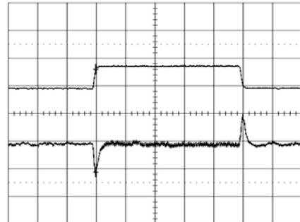
Output voltage response to load current step- change (7-15-7 A) at:
