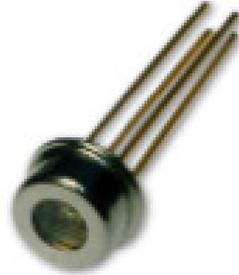
These products are high-performance 850nm VCSELs (Vertical Cavity Surface-Emitting Lasers) designed for high-speed data communications and packaged with a custom designed power monitor diode. The power monitor diode can be used with appropriate feedback control circuitry to set a maximum power level for the VCSEL. These combined features simplify design for high data rate communication and eye safety.
