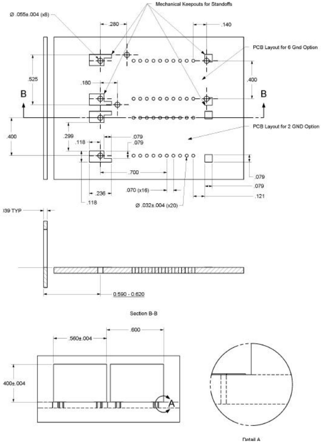
**Minimum Recommended Module-to-Module Spacing is 0.6 inches**
