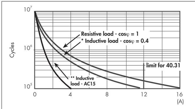
\* Inductive load -  $\cos\phi = 0.4$ : inrush current = rated current
