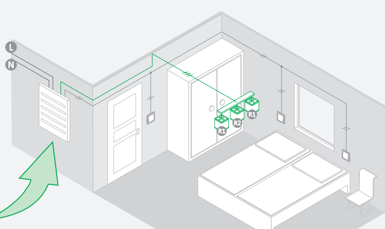
Example of a lighting system for controlling the light intensity by switching on sections R1 and R2 respectively
