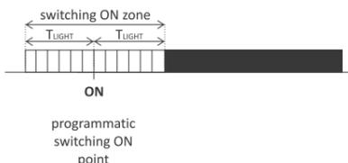
If in the selected switching zone the measured brightness level drops below the value set in parameter 6.6.4, switching-on will take place before the **ON** time. If the measured brightness level is greater than the value set in parameter 6.6.5, switching-on will take place after the **ON** time.
