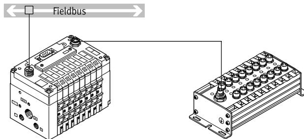
Fieldbus Direct is a system for the compact connection of a CPV or CPV-SC valve terminal to different fieldbus standards such as PROFIBUS and DeviceNet.
