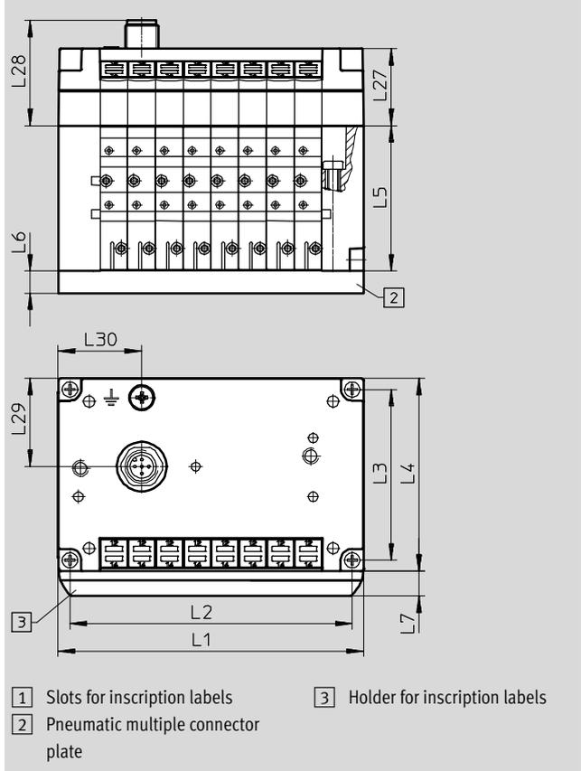
Valve terminal with installation system CPI
