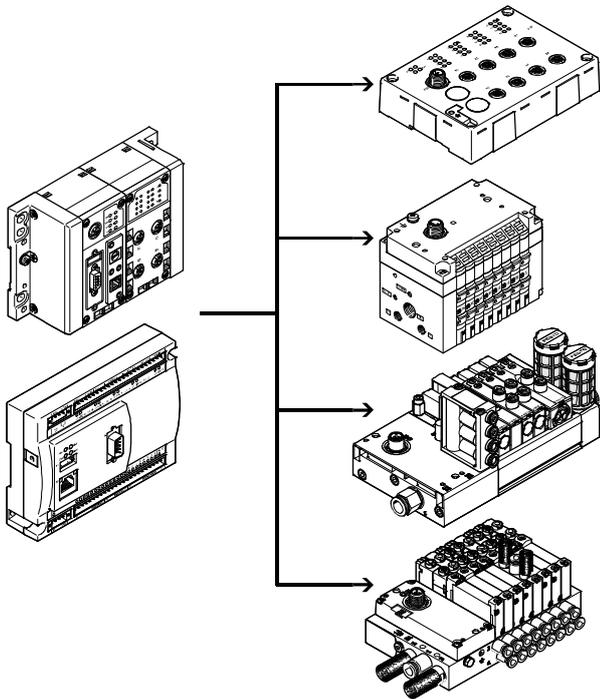
A CTEL system consists of the CTEL master and the devices with I-Port interface, which are connected together using special connecting cables. This permits a decentralised layout of the devices. This means that the valve terminals and I/O modules with I-Port interface (devices) can be mounted very close to the cylinders to be controlled. This reduces the length of the air supply lines used, which minimises flow losses and pressurisation and venting times.
