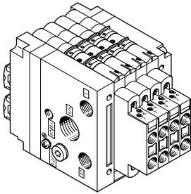
These valve extensions (vertical stacking) can be used to add further pneumatic functions to CPV valve terminals size 10 and 14:
