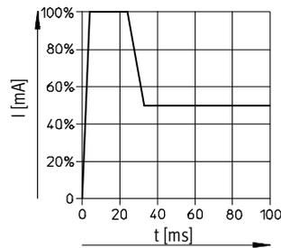
CPV10/14 valves are actuated by means of an integrated current reduction circuit, which reduces power consumption and heat build-up. This current reduction circuit is integrated in the basic electrical unit (multi-pin plug or fieldbus connection) or in the connecting cable.
