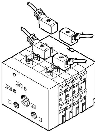
With an individual connection integration is only carried out in the pneumatic part, the solenoid valves are connected with individual cables.
