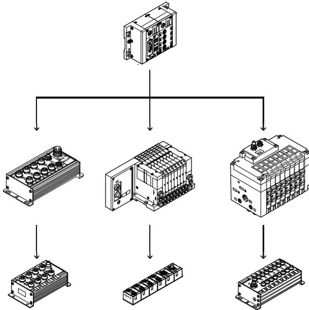
Valve terminals with CP connection are intended for connection to higher-order bus nodes or to control blocks. A bus node or control block also enables the connection of decentralised input/output units. The following bus protocols are supported:
