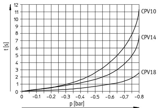
Suction capacity as a function of partial vacuum at P<sub>nominal</sub>
