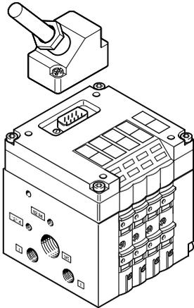
In addition to pneumatic integration, a multi-pin plug connection also provides integration of the electrical side and facilitates connection to the control cabinet and the valve terminal via a single cable.
