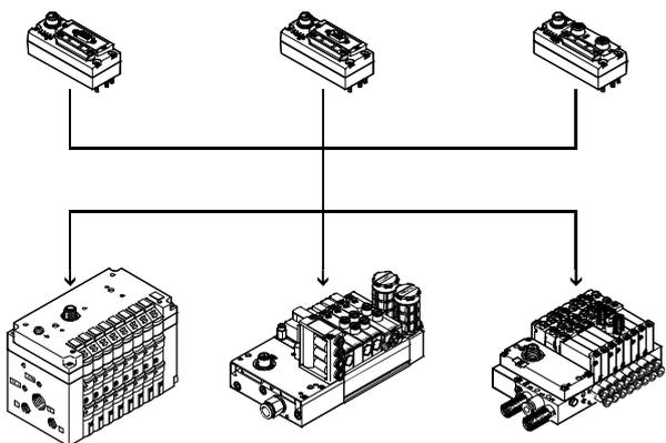
CTEU is a system for compact connection of a valve terminal to different fieldbus standards such as Profibus and DeviceNet.
