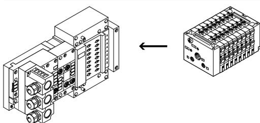
Adaptation of the CPV valve manifold to the input/output module ET200X/ET200pro from Siemens: the combination of the functional module of the ET200X/ET200pro and the pneumatic functions of the CPV valve manifold provides a highly integratable automation solution for systems using electrical and pneumatic drives with:
