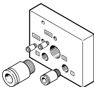
Example of an end plate: The diagram shows a left-hand end plate with external pilot air supply. The exhaust ports 3/5 and 82/84 can
