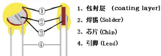
剖視圖 (sectional view)
