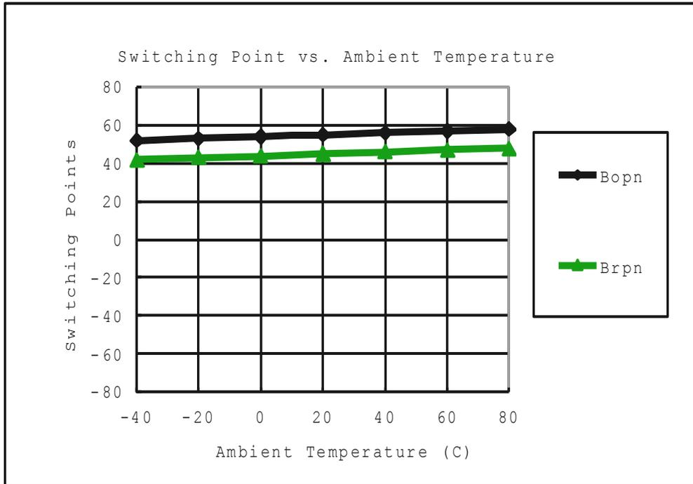
**Figure.4 Magnetic Switch Points Versus Ambient Temperature (VDD=2.7V)**
