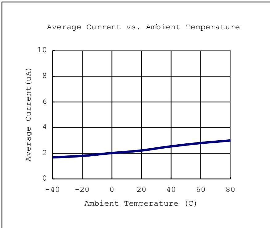
**Figure.7 Average Current Versus Ambient Temperature (VDD=2.7V )**
