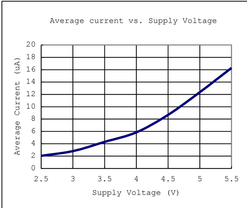
**Figure.6 Average Current Versus Supply Voltage ( Ta=25C degree)**
