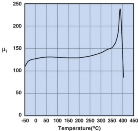
Measured on a 19/10/6mm toroid at 100kHz.
