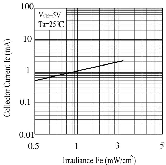
**Typical Electro-Optical Characteristics Curves**
