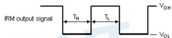
Fig.-2 Measuring Method
