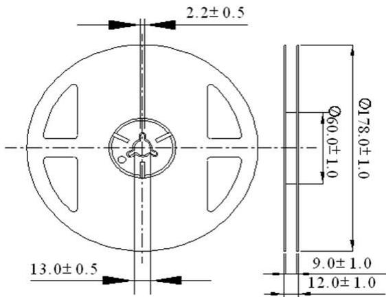
**Carrier Tape Dimensions: Loaded Quantity 4000 pcs Per Reel**
