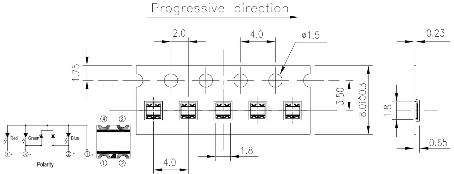
Note: The tolerances unless mentioned is  $\pm 0.1\text{mm}$  ,Unit = mm
