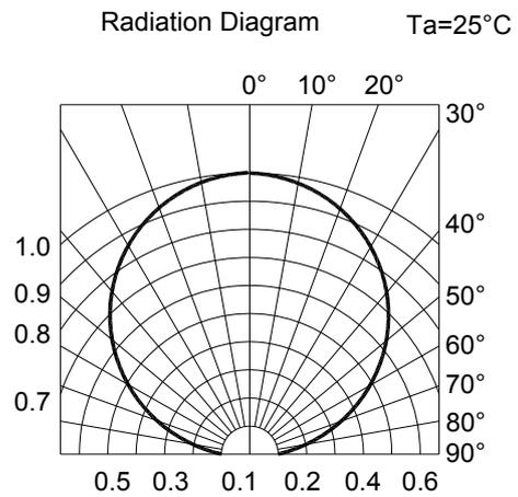
Typical Electro-Optical Characteristics Curves
