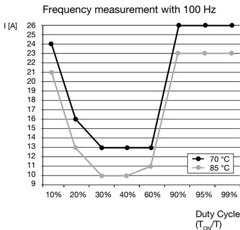
The max. load current depends on the load type. Please contact the manufacturer of the load if the limit values shown above are reached. E-T-A is able to test whether the relay works in the limit range.
