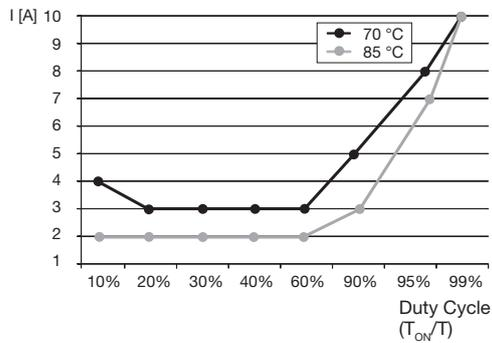
The max. load current depends on the load type. Please contact the manufacturer of the load if the limit values shown above are reached. E-T-A is able to test whether the relay works in the limit range.
