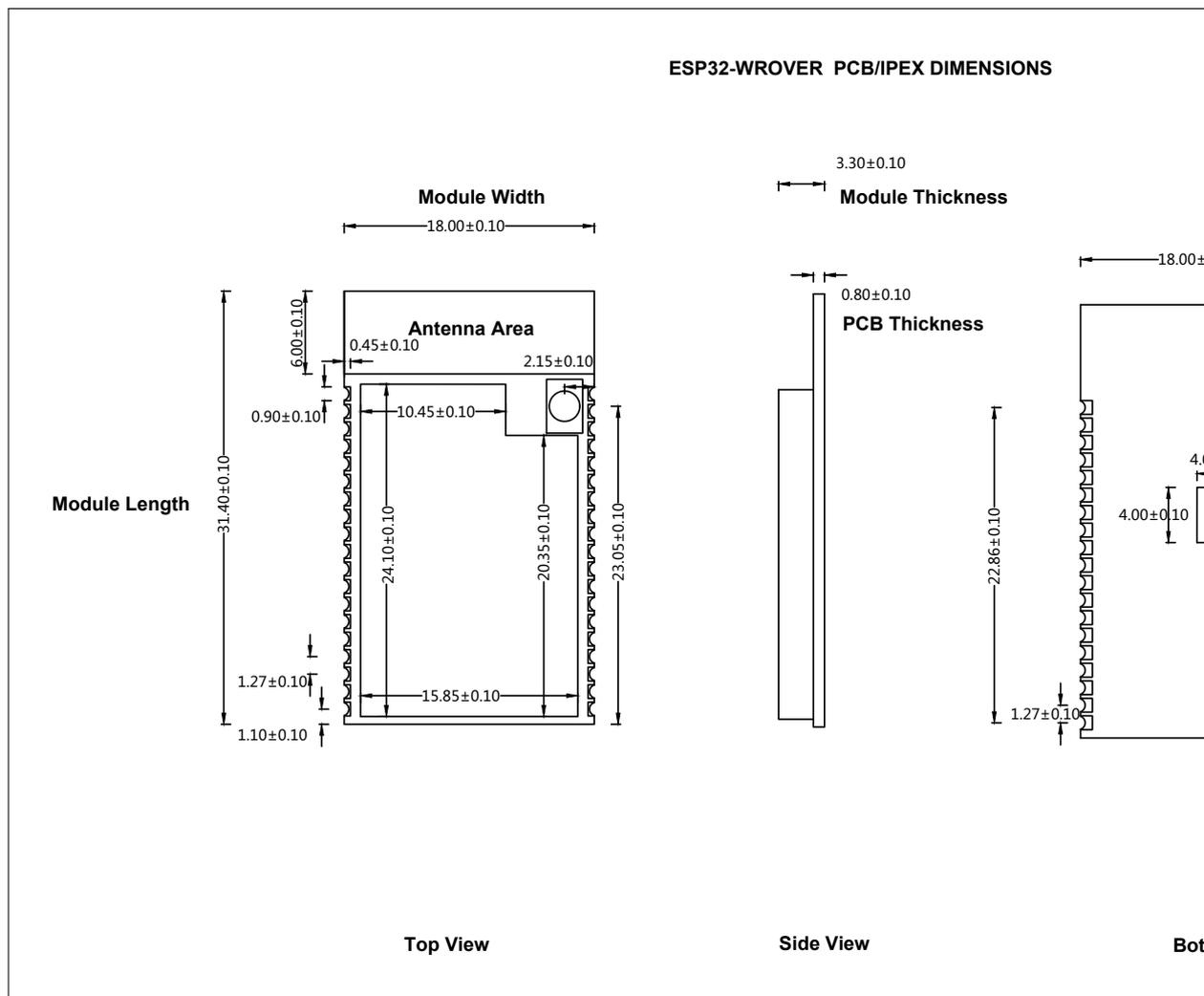
图 7: ESP32-WROVER (PCB/IPEX) 尺寸图
