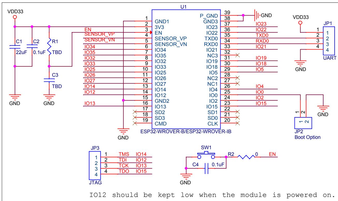
Figure 5: Peripheral Schematics
