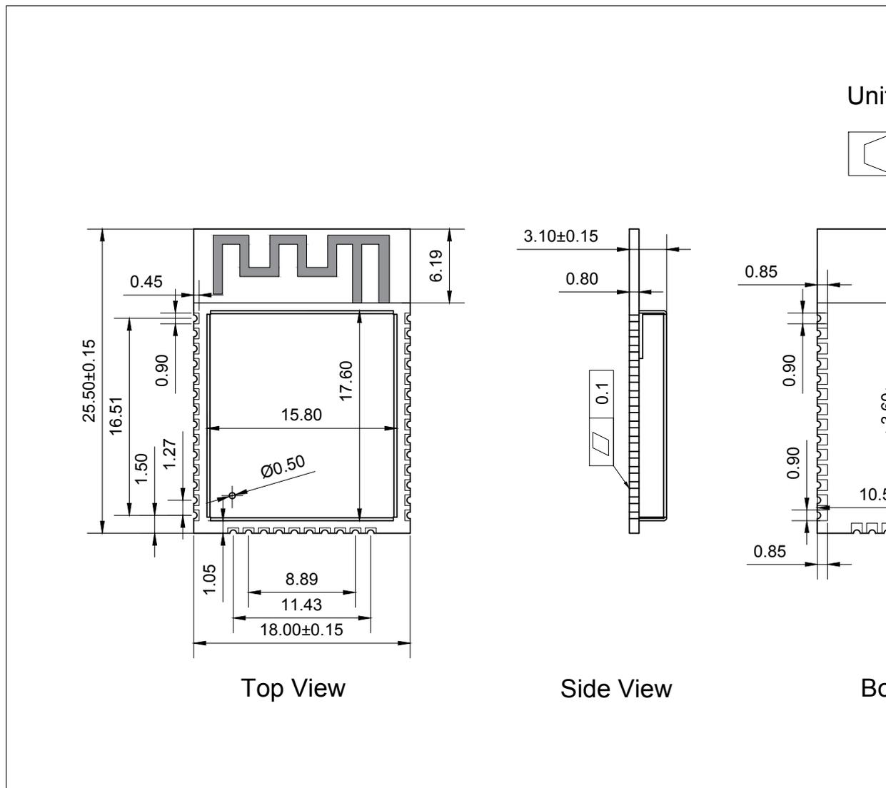
Figure 5: Physical Dimensions of ESP32-SOLO-1
