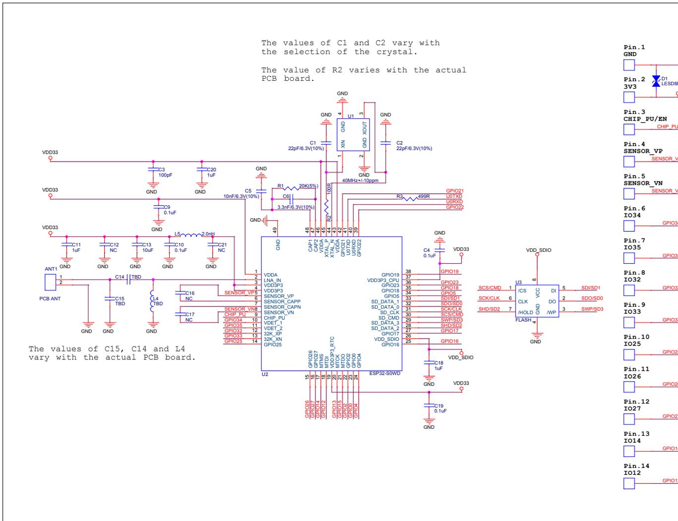
Figure 3: ESP32-SOLO-1 Schematics
