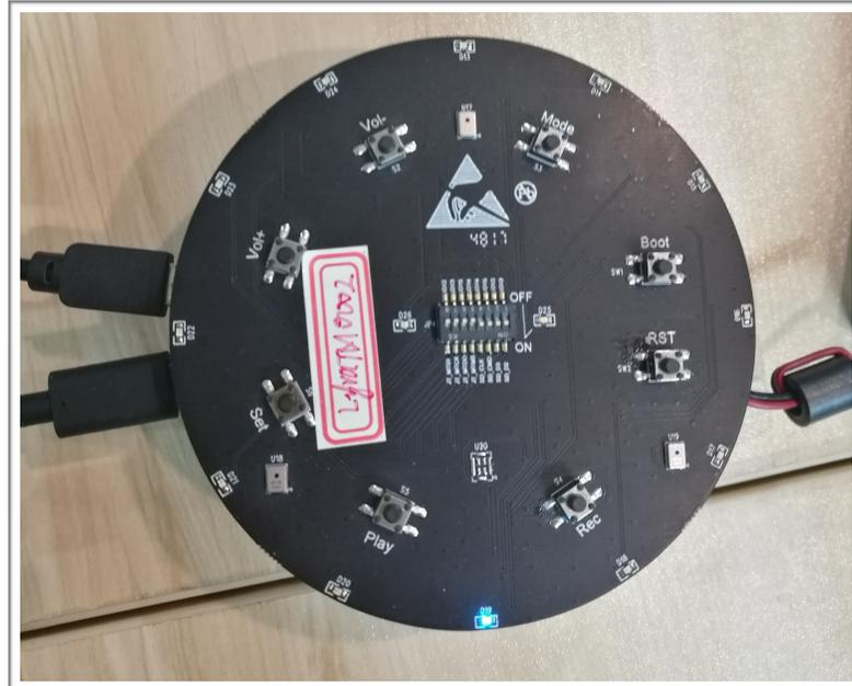
Figure 2-6. The LED Light on ESP32-LyraTD-MSC
