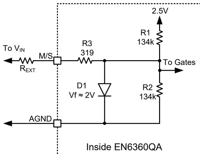
**Figure 7: Selection of R<sub>EXT</sub> to Connect M/S pin to V<sub>IN</sub>**
