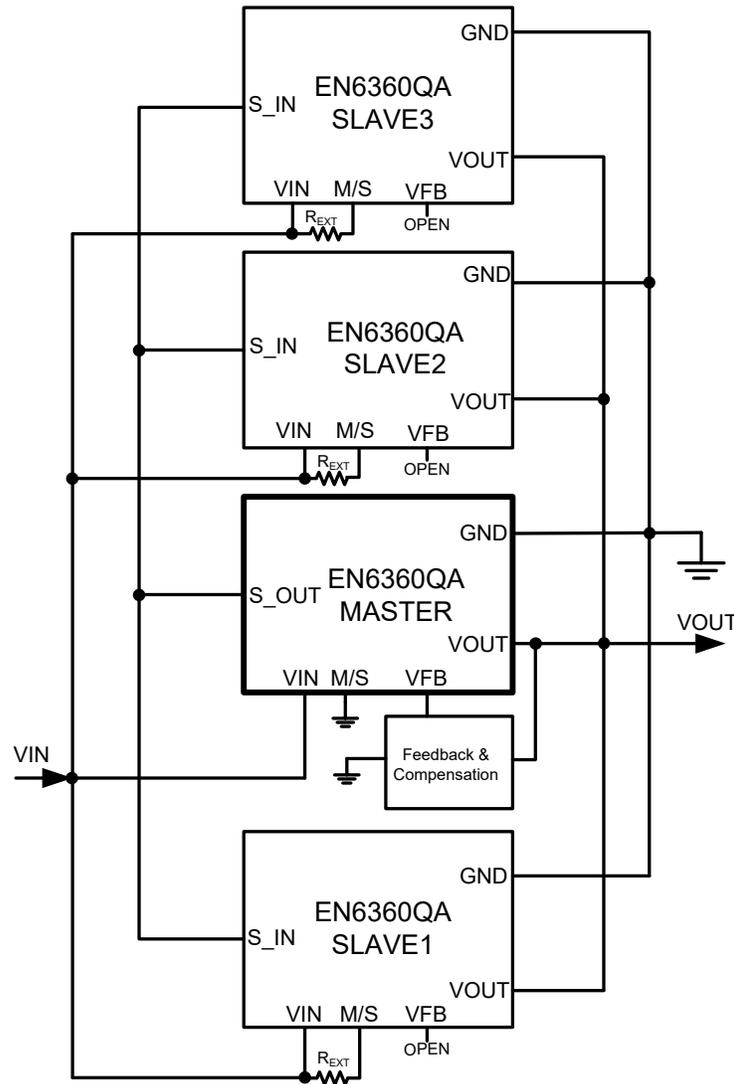
Figure 5: Master/Slave Parallel Operation Diagram POK Operation
