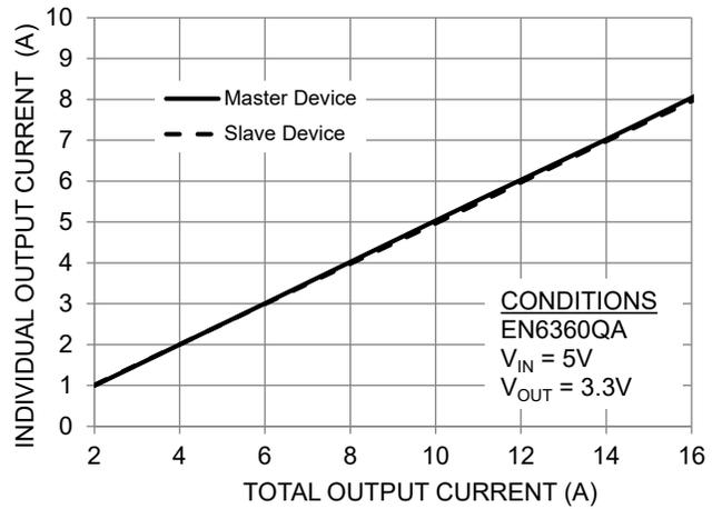
**Parallel Output Voltage vs. Output Current**
