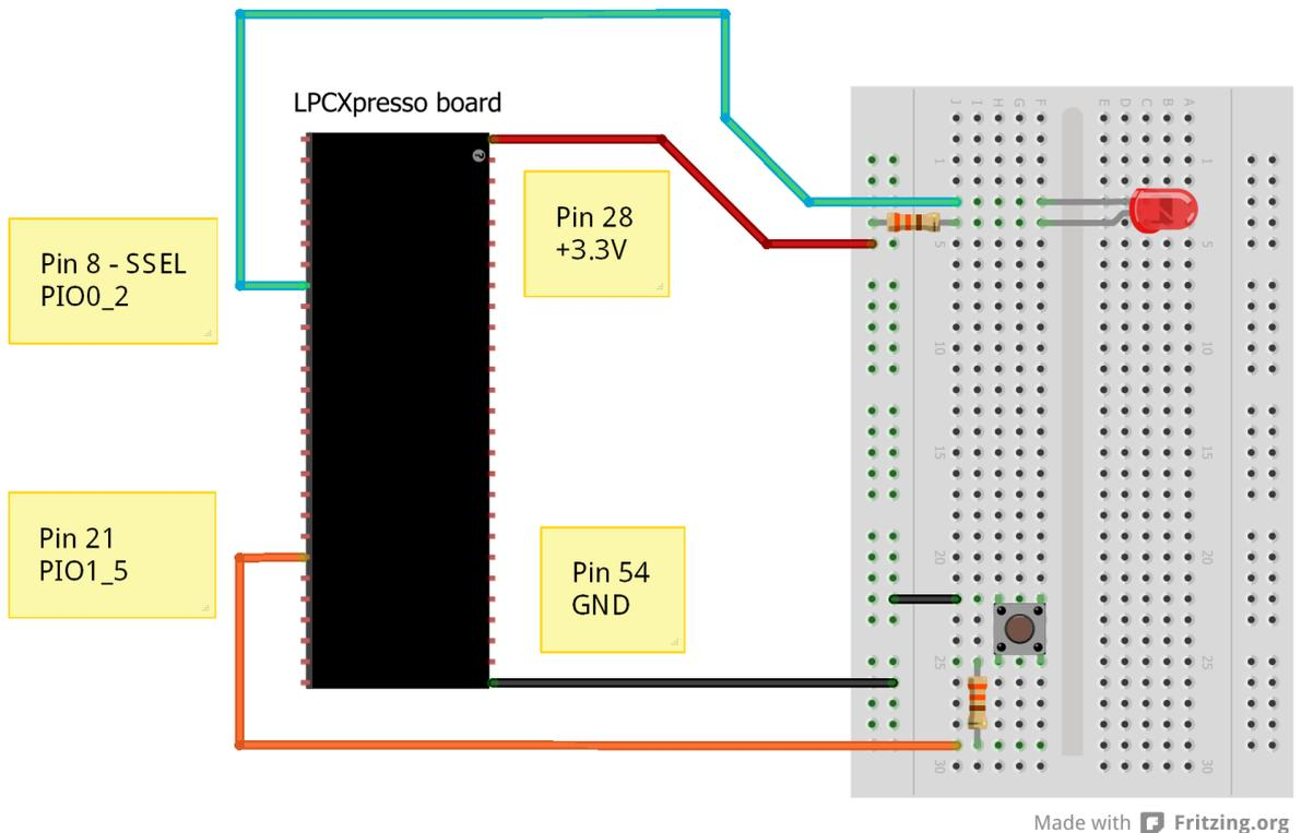
Figure 13 – Breadboard Connections for SW2 and LED
