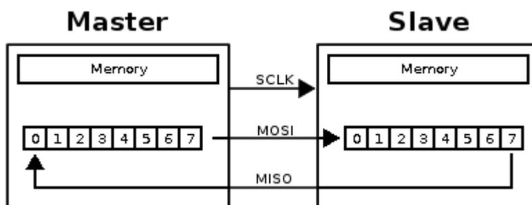
Figure 47 – SPI Master and Slave Connection
