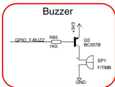
Figure 15 – Buzzer on Schematic Page 4
