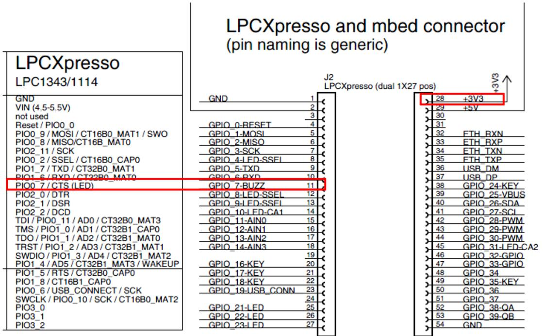
Figure 16 – Signal GPIO\_7-BUZZ on Schematic Page 2
