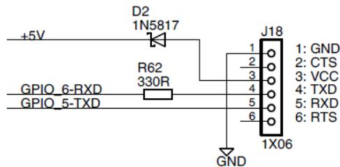
Figure 58 – J18, D2 and R62 on Schematic Page 7
