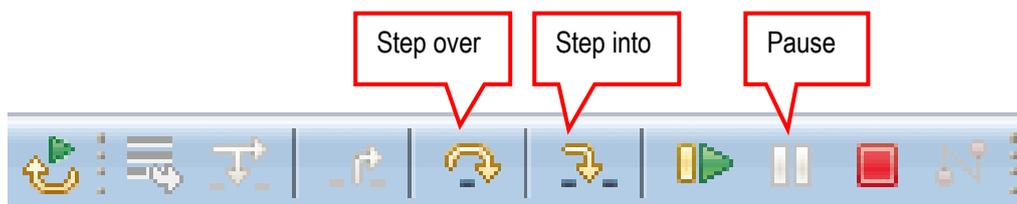
Figure 10 – LPCXpresso IDE Step Over/Into Buttons
