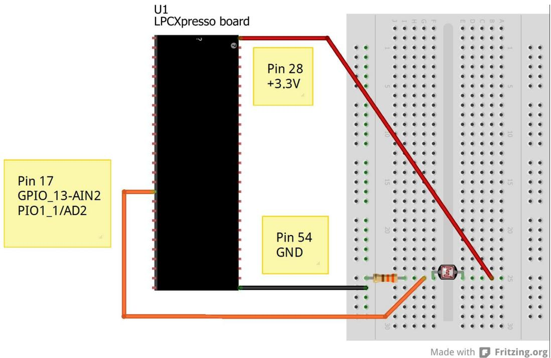
Figure 26 – Breadboard Connections for Light Sensor R24
