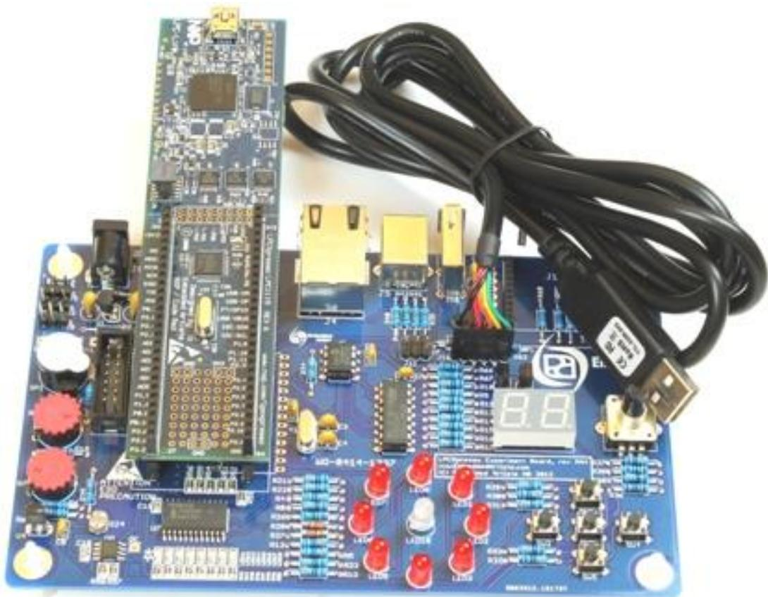
Figure 59 – LPCXpresso Experiment Kit PCB with UART-to-USB Cable
