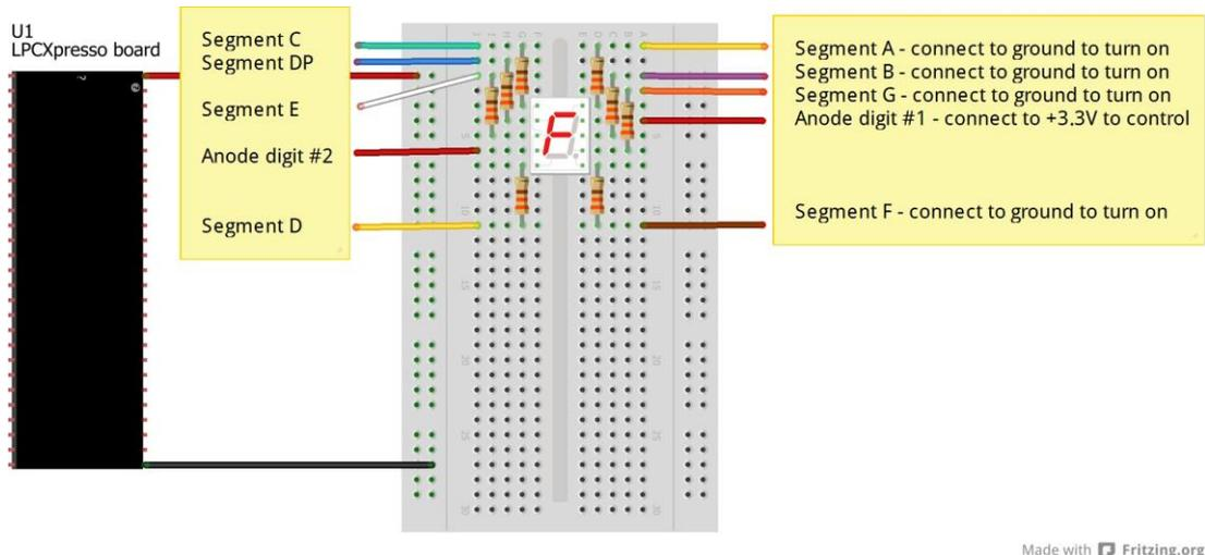
Figure 35 – Breadboard Connections for 7-segment Display Testing
