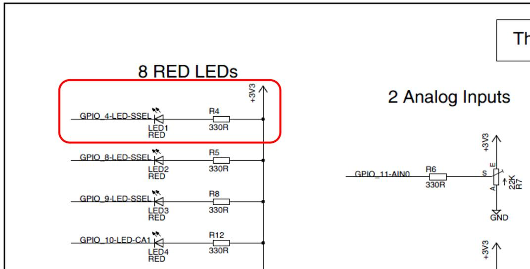
Figure 4 – LED1 on Schematic Page 4
