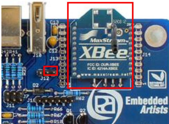
Figure 64 – XBee® Module Mounted in J15
