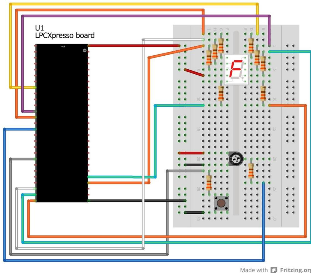
Figure 36 – Breadboard Connections for 7-segment Display
