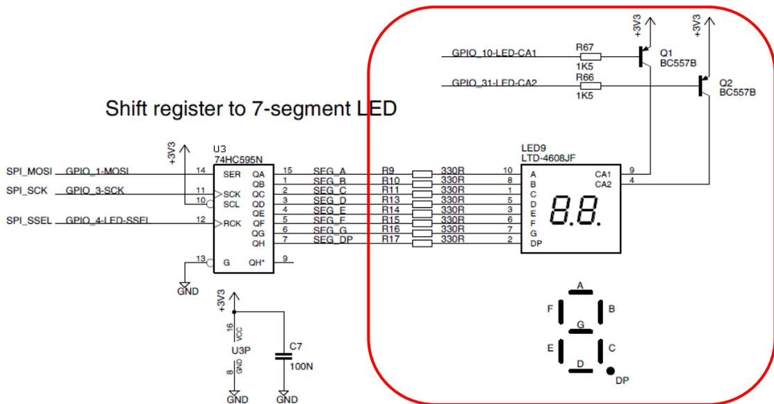
Figure 38 – 7-segment Display, LED9, on Schematic Page 4
