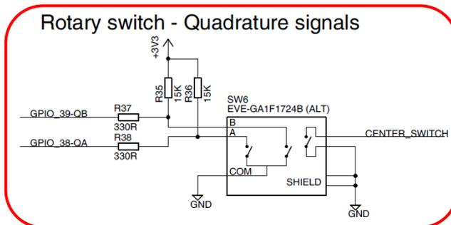
Figure 19 – Quadrature Encoder (SW6) on Schematic page 5
