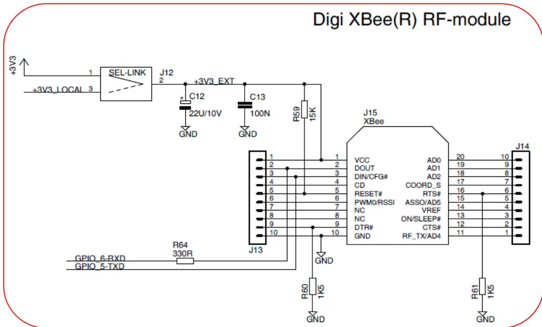
Figure 63 – RF Module Interface on Schematic Page 7
