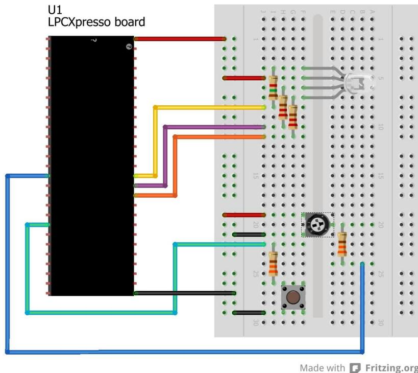
Figure 31 – Breadboard Connections for RGB-LED Experiments
