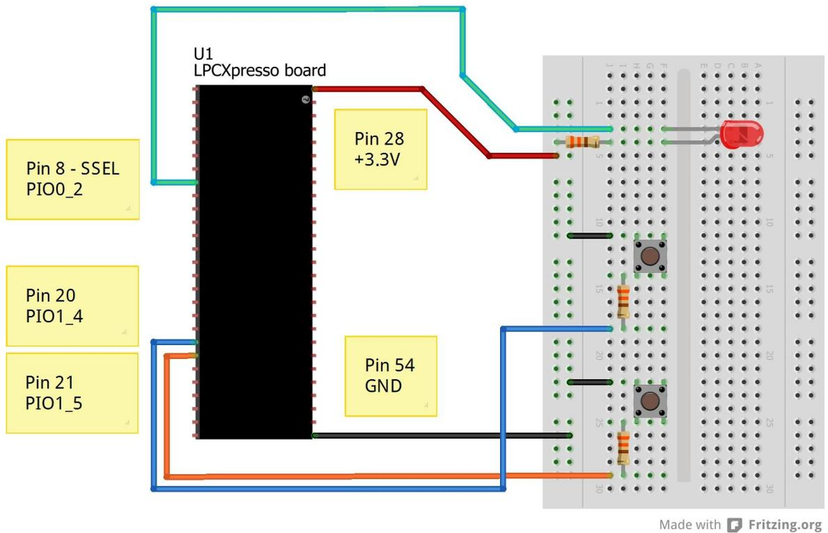
Figure 14 – Breadboard Connections for SW2, SW3 and LED
