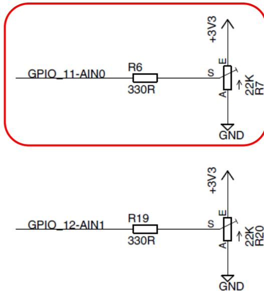
Figure 23 – Trimming Potentiometer on Schematic Page 4
