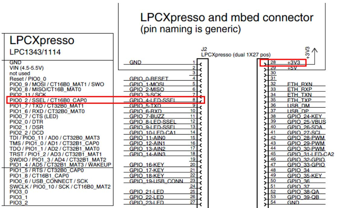
Figure 5 – Signal GPIO\_4-LED-SSEL on Schematic Page 2
