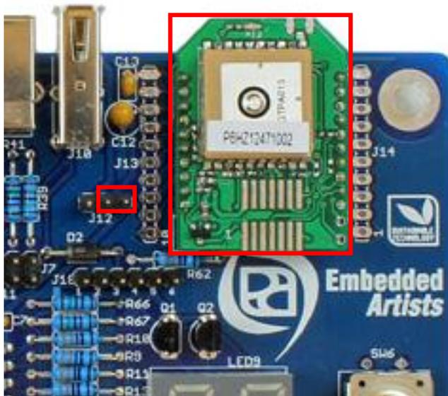
Figure 65 – GPS Module Mounted in J15
