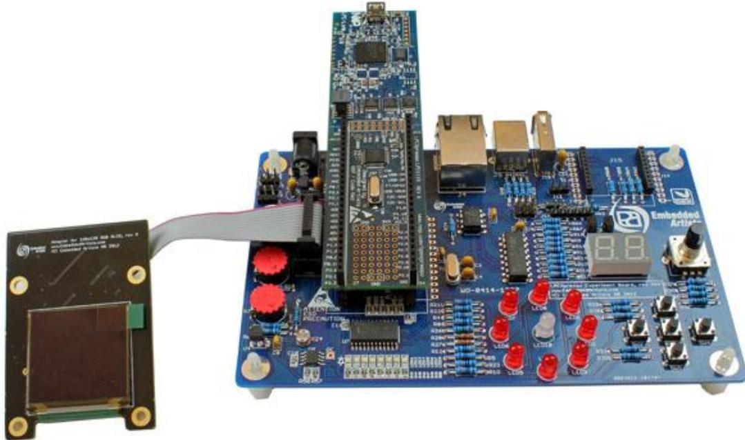
Figure 68 – 1.5 inch RGB OLED Connected via Serial Expansion Connector
