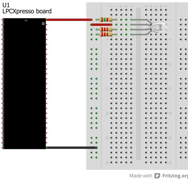
Figure 30 – Breadboard Connections for RGB-LED Testing
