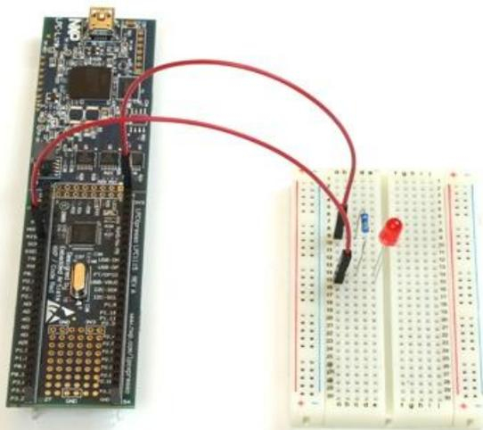
Figure 7 – Breadboard Connections for LED1 (real photo)
