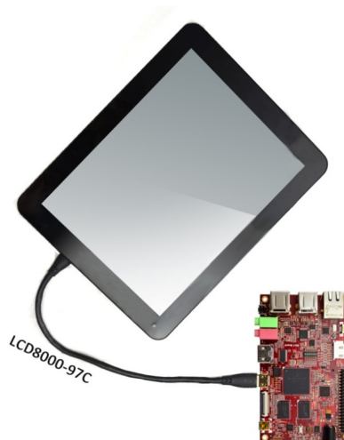
Figure 1 Connections between RIoTboard and LCD8000-97C
