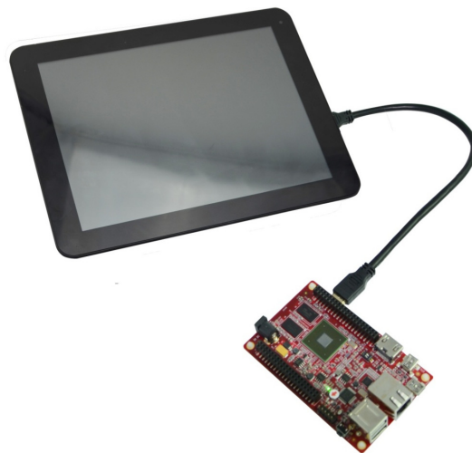
Figure 6 Connection between MarS Board and LCD8000-97C
