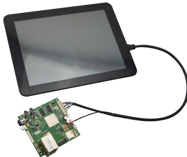
Figure 4 Connections between SABRE Lite and LCD8000-97C
