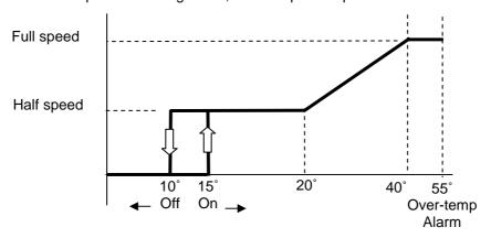
Each fan may have a different profile using either thermistor as configured.
