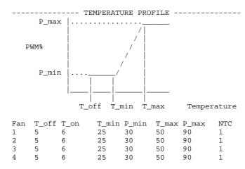
Type "1" to "4" to select Fan or Space to exit without changing Type "m" to enable Multi Point Profile or Space to exit without changing
