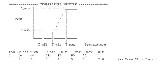
Type "4" to change the PWM Output at the Bottom of Proportional Control Band and below, display will be as shown:
