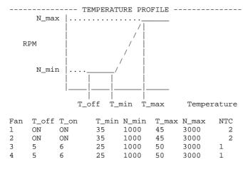
In this operating mode the Controller output sets the fan RPM (Closed Loop control). The fan speed control PWM output will be continuously adjusted to bring the measured fan RPM to the set value.
