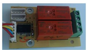
The interface used is compatible with the ebm-papst "EC Matrix" control bus, support for other EC-Matrix boards possible, contact ebm-papst.
