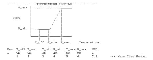
Type "5" to change the Temperature at the Top of Proportional Control Band, display will be as shown:
