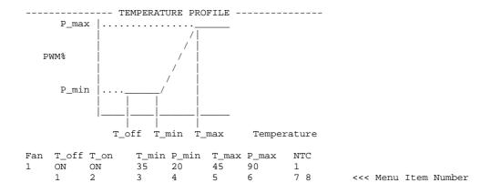
Type "6" to change the PWM Output at the Top of Proportional Control Band and above, display will be as shown:
