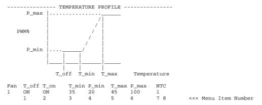
Type "8" to change the NTC Thermistor 2 used setting, if both thermistors selected then speed will be set by whichever of NTC Thermistor 1 or NTC Thermistor 2 is hottest. Display will be as shown:
