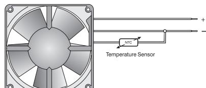
The temperature sensor for controlling the motor speed is not included in the scope of delivery.
