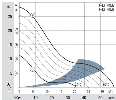
Air performance measured according to: ISO 5801. Installation category A, without contact protection.
