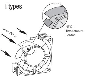
The temperature sensor (NTC resistor) for controlling the motor speed is positioned in the fan hub directly in the air flow.
