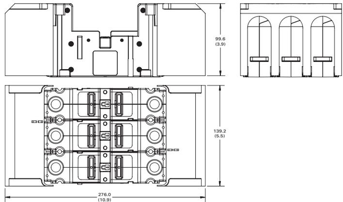
3-pole ganged 400 A holder with installed shroud
