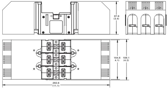
3-pole ganged 200 A holder with installed shroud
