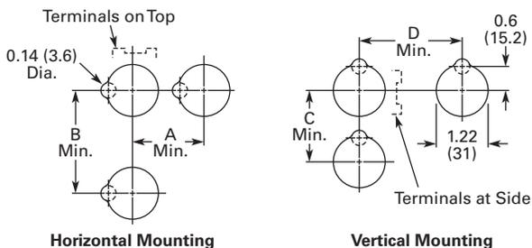
Horizontal mounting means terminals are located top and bottom of contact block. Vertical mounting means terminals are left and right of contact block. This allows close spacing of adjacent operators with easy access to terminals.
