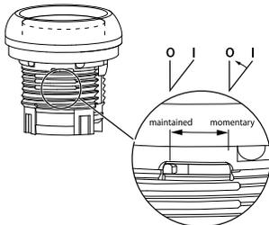
**Note:** This pilot device features a selectable function switch that enables the device to be set to either maintained or momentary operation.
