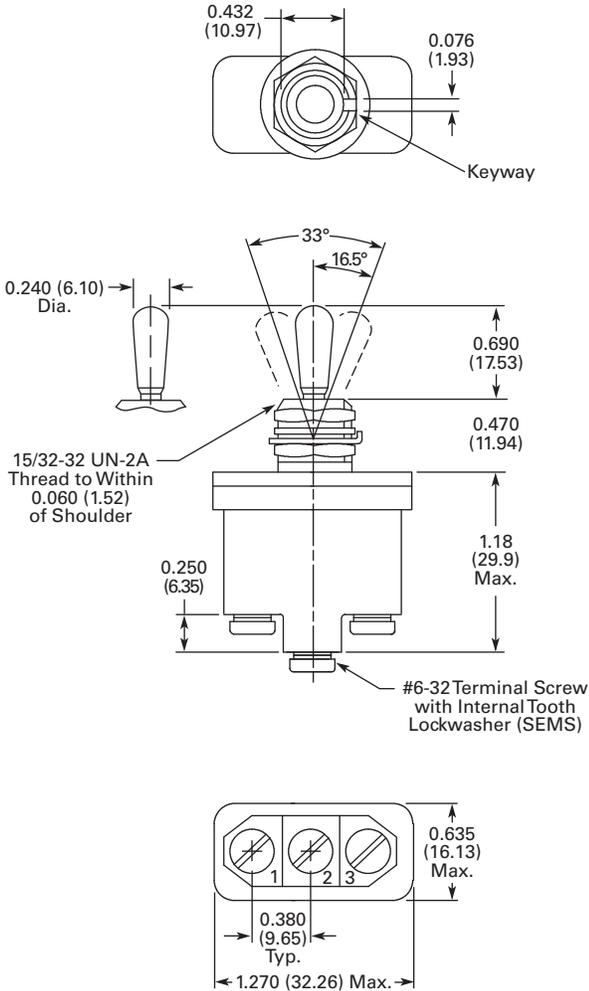
**Two-Pole Molded-In Screw Terminal E10E Series**
