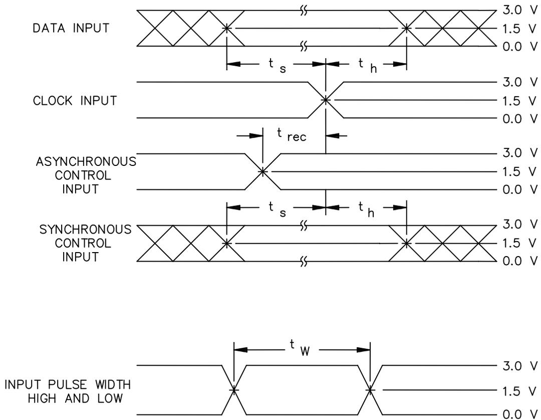
FIGURE 5. Switching waveforms and test circuit.
