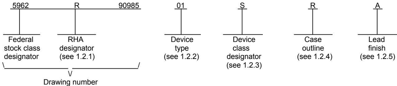
1.2.1 RHA designator. Device classes B, S, Q, and V RHA marked devices meet the MIL-PRF-38535 specified RHA levels and are marked with the appropriate RHA designator. Device class M RHA marked devices meet the MIL-PRF-38535, appendix A specified RHA levels and are marked with the appropriate RHA designator. A dash (-) indicates a non-RHA device.
