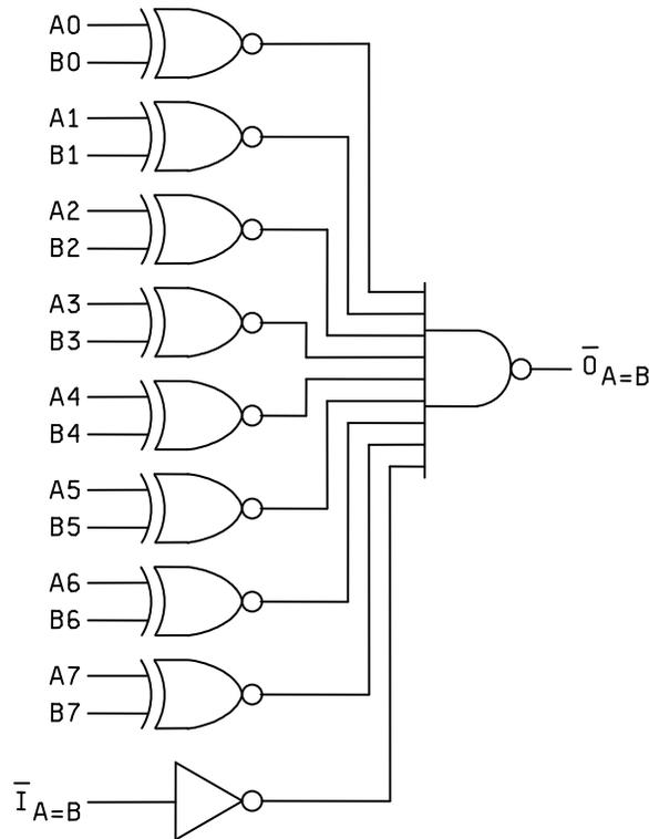
FIGURE 3. Logic diagram.
