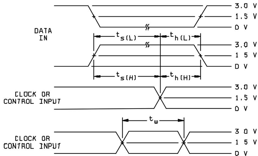
SETUP TIME, HOLD TIME AND PULSE WIDTHS
