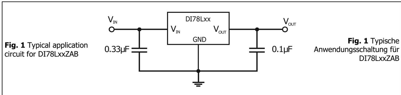
**Fig. 1** Typical application circuit for DI78LxxZAB
