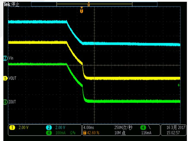
Over-Load to No-Load Recovery Response
