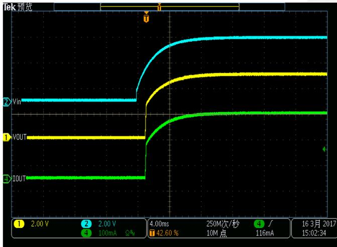
No-Load to Over-Load Transient Response
