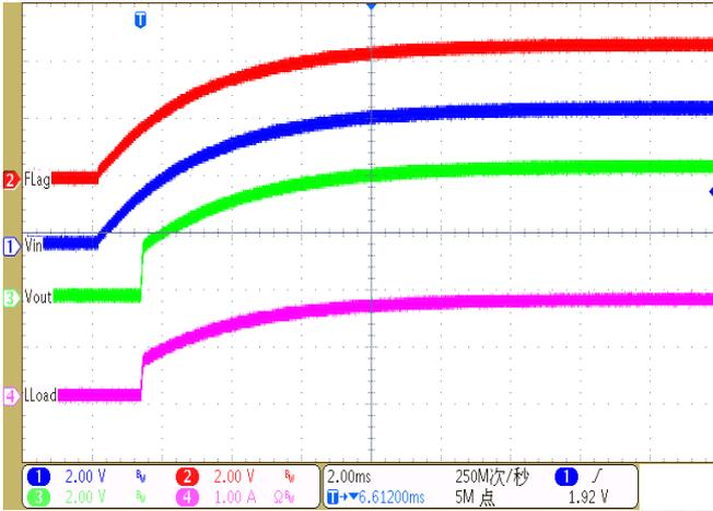
Power off (Vin=5V, RLoad=2.5ohm)
