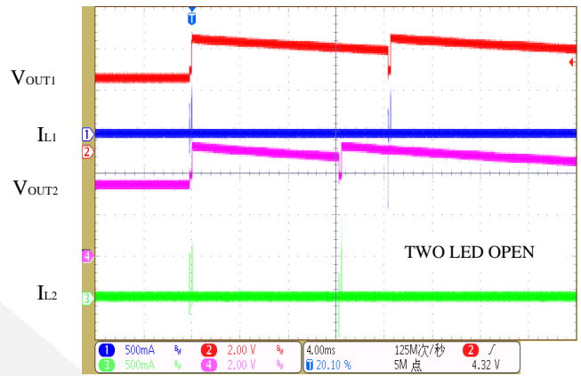
LED Open Circuit Protection
