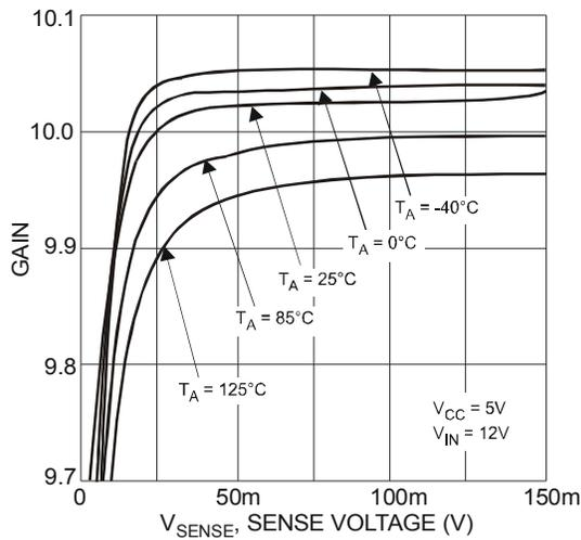
Fig. 9 Differential gain
