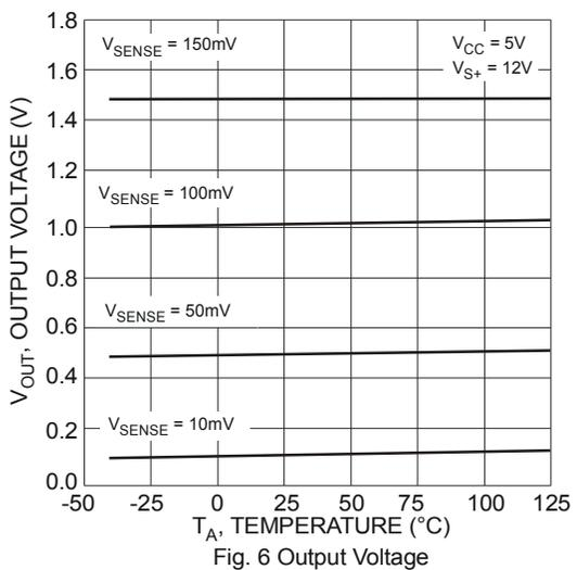
**Typical Characteristics** (cont.) (@  $V_{IN} = 12V$ ,  $V_{CC} = 5V$ ,  $V_{SENSE+} = 12V$ ,  $V_{SENSE} = 100mV$ ,  $T_A = +25^\circ C$ , unless otherwise specified.)
