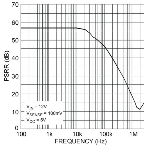
Fig. 19 Supply Rejection
