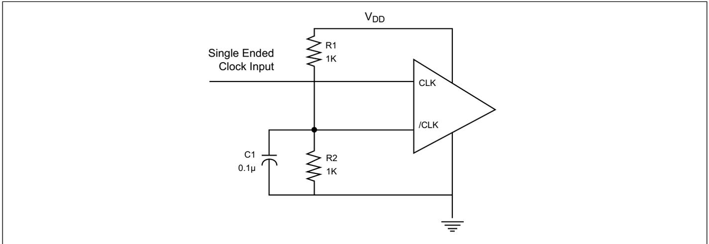
**Figure 1. Single-ended Input to Differential Input Device**
