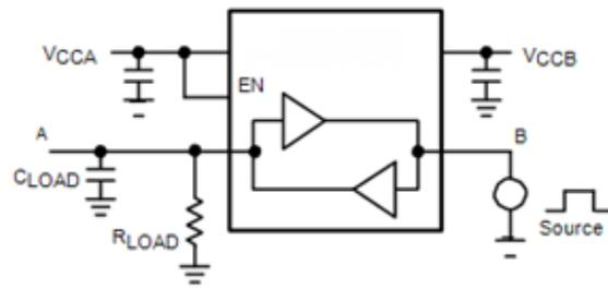
Figure 2. Driving B Test Circuit
