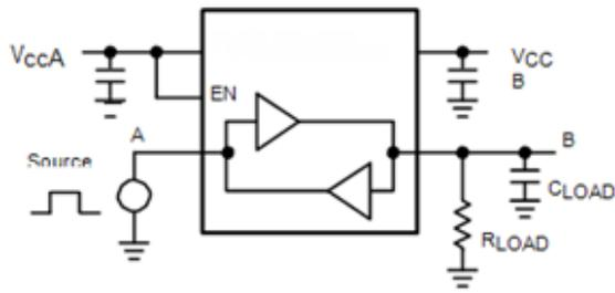
Figure 1. Driving A Test Circuit
