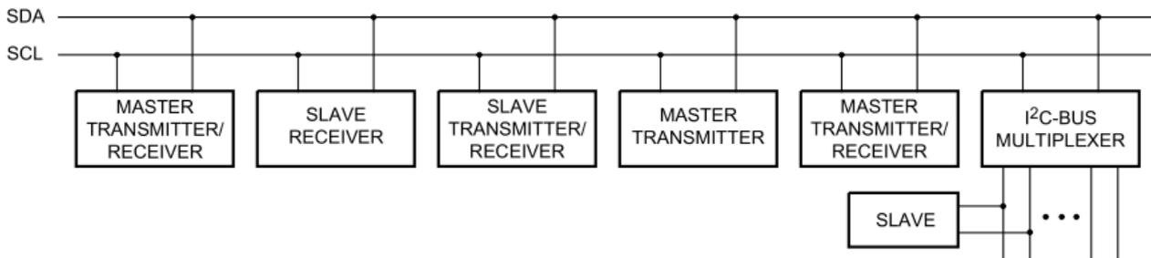
Figure 9. System Configuration
