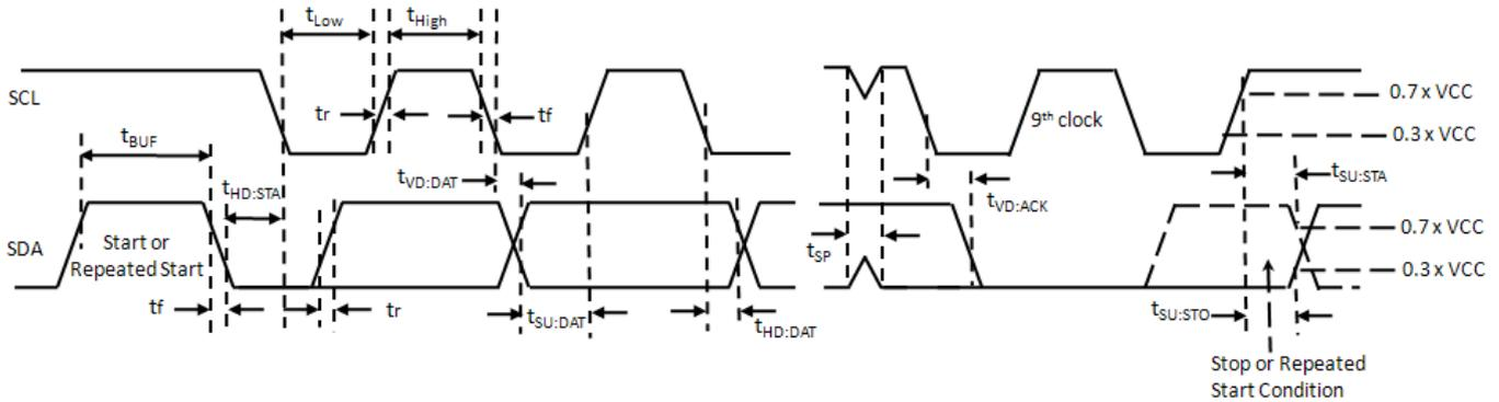
Figure 2. Definition of timing on the I2C-bus
