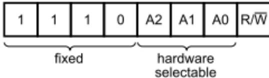
Figure 4: Device address
