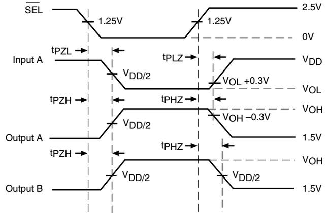
**Voltage Waveforms Propagation Delay Times**
