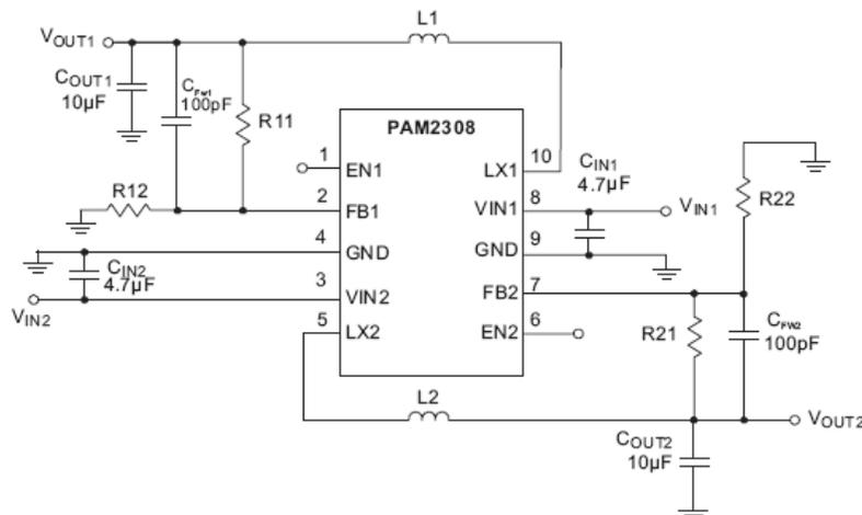
$$V_{OUTx} = V_{REF} \left( 1 + \frac{R_{x1}}{R_{x2}} \right)$$
