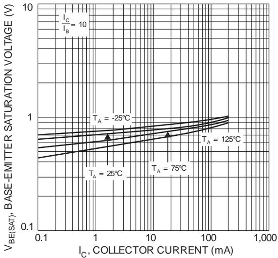
Fig. 3 Typical Base-Emitter Saturation Voltage vs. Collector Current
