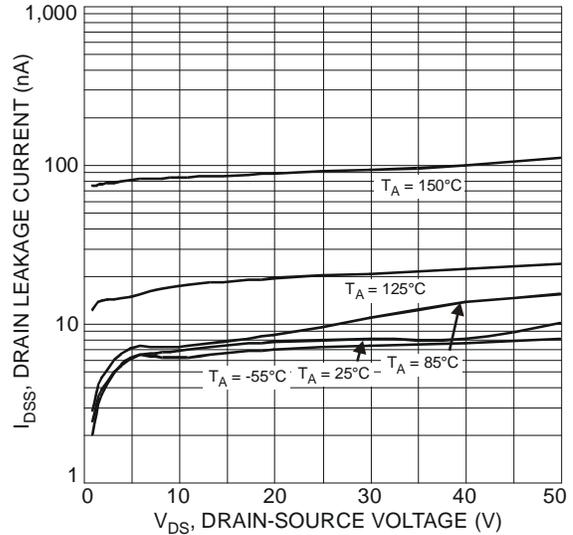
Figure 8. Typical Drain-Source Leakage Current vs. Voltage
